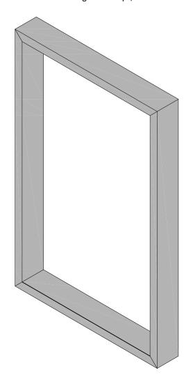
4) Maximum centres can now be determined by cross referencing shroud size vs. wind zone on the table of the appropriate subtrate/cladding drawing. The correct bracket size will also be detailed there. Please ensure to position one bracket per corner and wherever possible use side (vertical) brackets as they are preferred for waterproofing.
