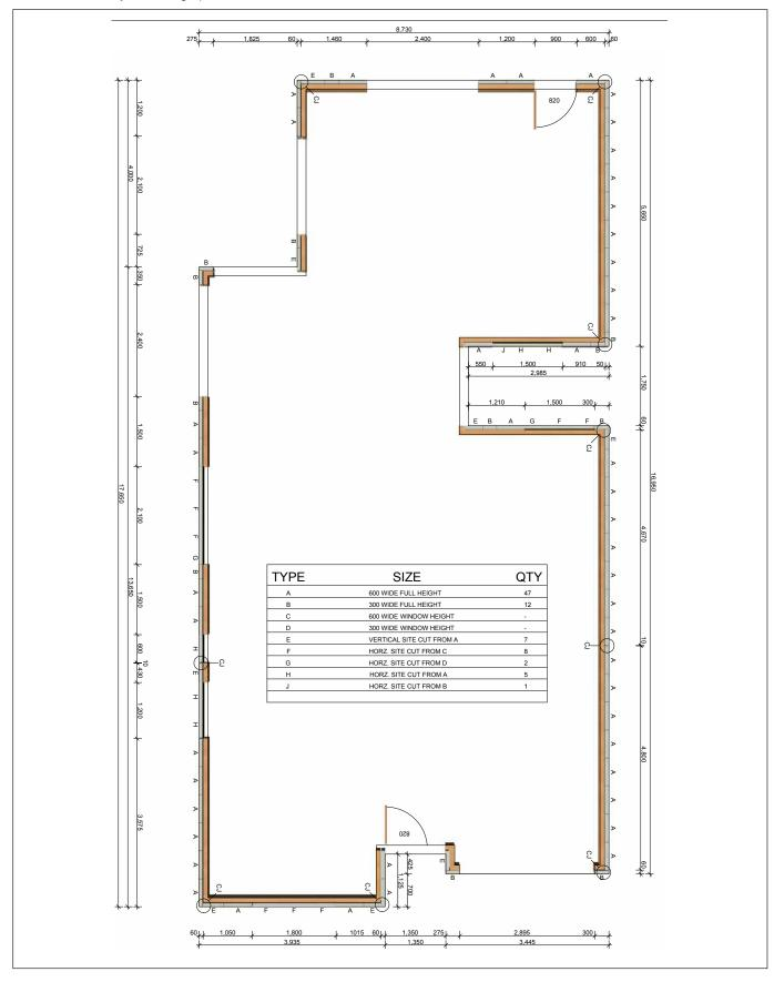
1. At corners, PowerPanel<sup>50</sup> panels can be laid out at 300mm multiples in one direction and 300mm multiples + 60mm in the other direction 2. Width of PowerPanel<sup>50</sup> panels may vary + or - 1.5mm
