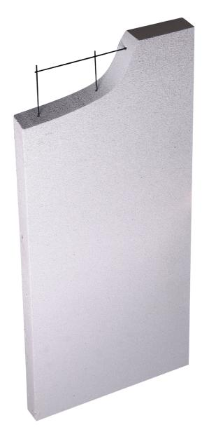
At the heart of the Hebel residential external wall system is the Hebel PowerPanel<sup>50</sup> - a 50mm thick, steel reinforced building panel made from AAC (Autoclaved Aerated Concrete) supplied in lengths of 2400mm with standard widths of 600mm.
