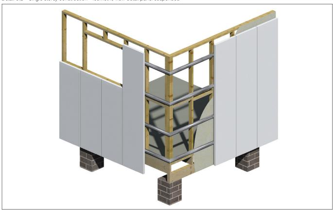
Detail 3.3 - Single storey construction - hip roof elevation
