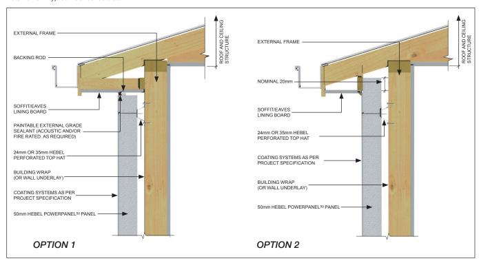
Detail 3.26 - Typical roof eaves detail (no eave overhang)
