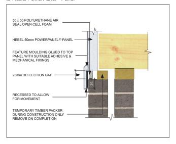
Detail 3.41 - Typical vertical control joint
