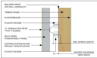
NOTE: When positioning the stud frames allow 5-7mm extra cavity width for the sheet bracing between Top Hat and timber stud.
