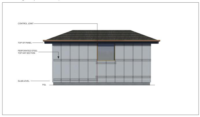
Detail 3.4 - Single storey construction - gable end elevation
