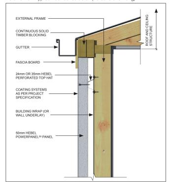
Detail 3.27 - Typical roof/parapet wall detail
