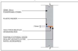
Top view - Horizontal control joint
