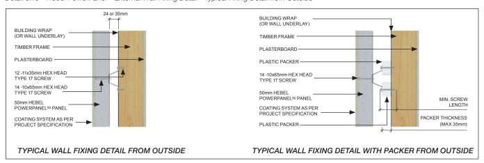
NOTE: When positioning the stud frames allow 5-7mm extra cavity width for the sheet bracing between Top Hat and timber stud.
