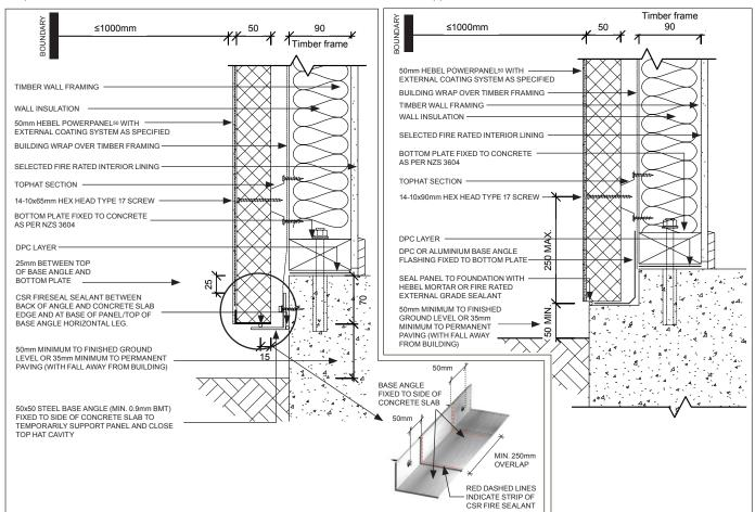
Fig. 2.3-50mm PowerPanel50 Boundary Wall - Typical Eaves Detail
