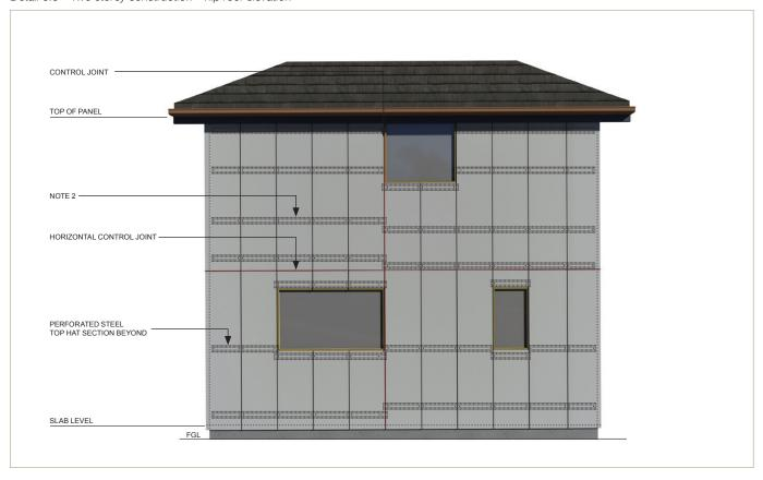
Detail 3.9 - Two storey construction - gable end elevation
