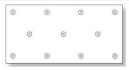
Suggested Layout of fasteners on a 1200 x 2400mm sheet.
