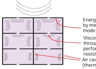
Energy dissipation by membrane mode (loss factor) Viscous loss through perforation (flow resistance) Air cavity effect (thermo viscous boundary layers) Reflected sound Acoustical Material Wall
