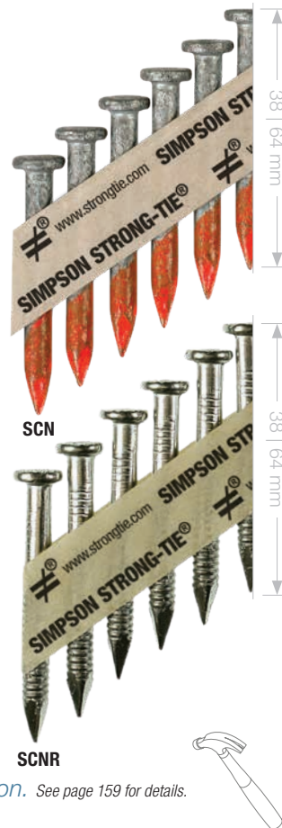
Annular threads create an interlock between the shank of the nail and the wood, providing superior holding power. Generally considered the nail type with the best withdrawal resistance.
