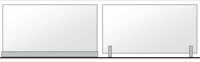
Top fixed mechanical channel. Concrete or timber fixing available. Powder coated to suit.
