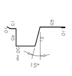
(Dimensions are indicative only) Turn down end of head flashing
