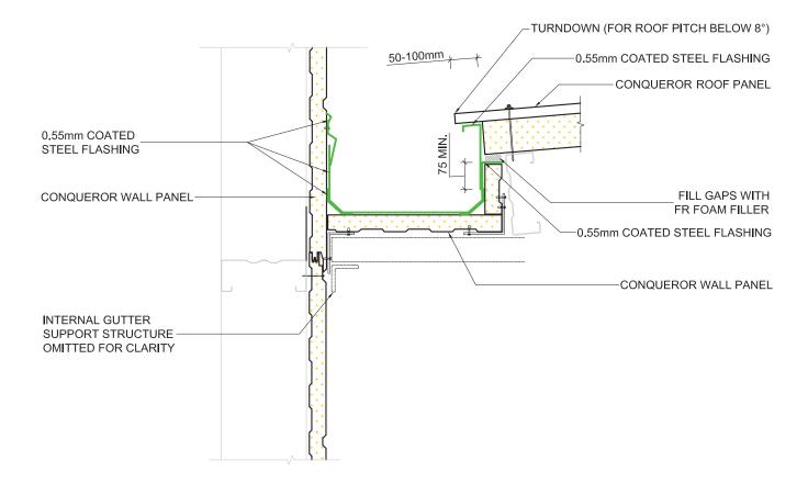
NOTE: ALL FLASHING SEALED WITH GUN GRADE BUTYL SEALANT
