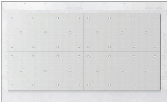
Figure 1.2. Board joints aligned. Fastener pattern (11 fixings per board)
