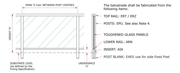
THIS SPECIFICATION IS BASED ON THE ATTACHMENT OF THE BALUSTRADE BEING IN ACCORDANCE WITH ONE OF THE STANDARD SIDE FIXING SPECIFICATIONS CONTAINED ON PAGES 32–37. REFER TO UNEX SYSTEMS FOR NON-STANDARD FIXING METHODS.
