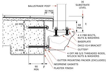
\*Gutter and associated clips flashings and packers are not supplied by the Unex Systems or the balustrade installer. Additional flashings may be required for water deflection in some cases. Gutter profile illustrated is "150mm O/G" from "Continuous Spouting", for more information on supplier visit www.cspout.co.nz. Other gutter profiles may be used. We do not recommend using copper gutters with this detail.
