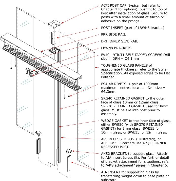
Note: Side rail height shall not be less than the minimum barrier height, as required in F4/AS1.
