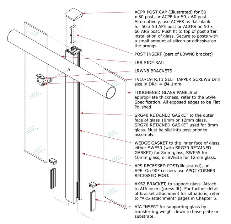
Note: Side rail height shall not be less than the minimum barrier height, as required in F4/AS1.
