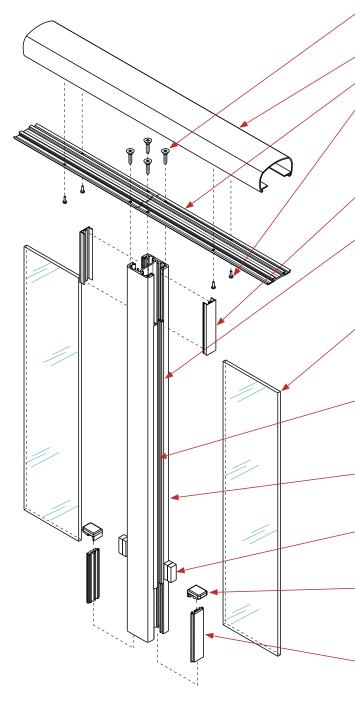
FV10-19 SCREWS. 4 per post. Drill size = Ø5.5mm.
