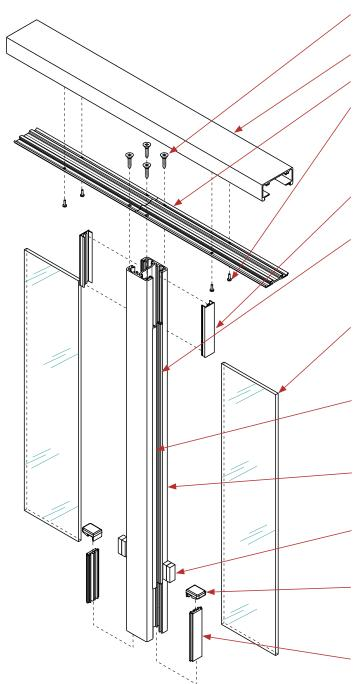
FV10-19 SCREWS. 4 per post. Drill size = Ø5.5mm.
