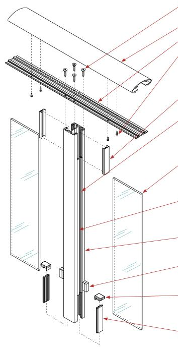
FV10-19 SCREWS. 4 per post. Drill size =  $\emptyset$ 5.5mm.
