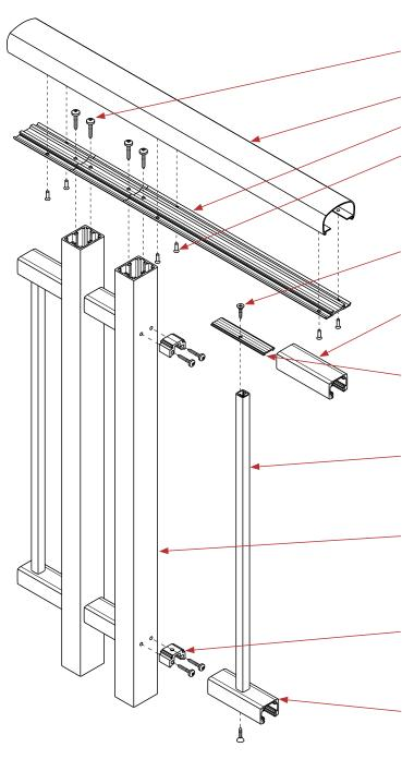
FT10-25.T1 SCREWS. 2 per post. Drill size =  $\emptyset$ 5.5mm.
