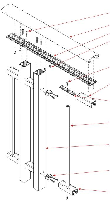
FT10-25.T1 SCREWS. 2 per post. Drill size = Ø5.5mm.
