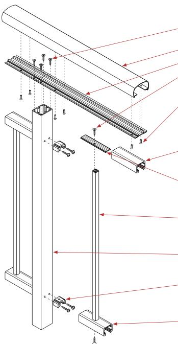
FV10-19.T1 SCREWS. 4 per post. Drill size =  $\emptyset$ 5.5mm.
