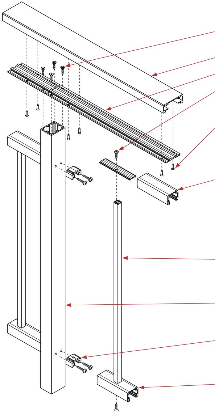
FV10-19.T1 SCREWS. 4 per post. Drill size = Ø5.5mm.
