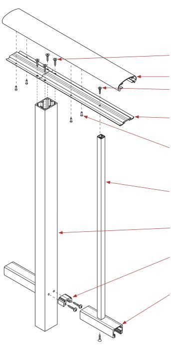
FV10-19.T1 SCREWS. 4 per post. Drill size = Ø5.5mm.
