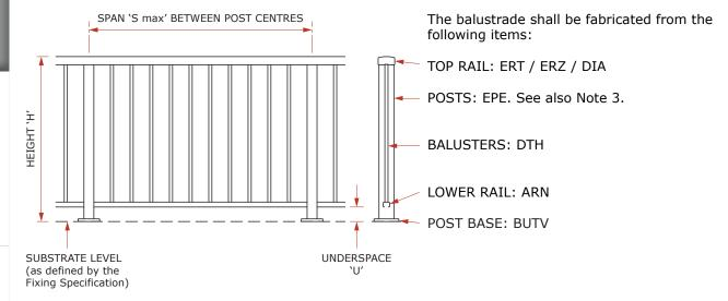
THIS SPECIFICATION IS BASED ON THE ATTACHMENT OF THE BALUSTRADE BEING IN ACCORDANCE WITH ONE OF THE STANDARD TOP FIXING SPECIFICATIONS CONTAINED ON PAGES 32-37. REFER TO UNEX SYSTEMS FOR NON-STANDARD FIXING METHODS.
