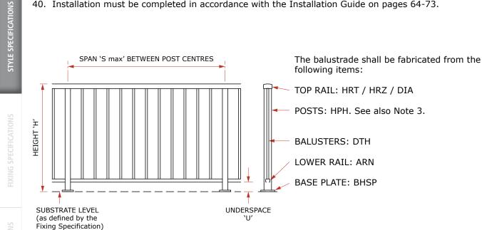
THIS SPECIFICATION IS BASED ON THE ATTACHMENT OF THE BALUSTRADE BEING IN ACCORDANCE WITH ONE OF THE STANDARD TOP FIXING SPECIFICATIONS CONTAINED ON PAGES 26–31. REFER TO UNEX SYSTEMS FOR NON-STANDARD FIXING METHODS.
