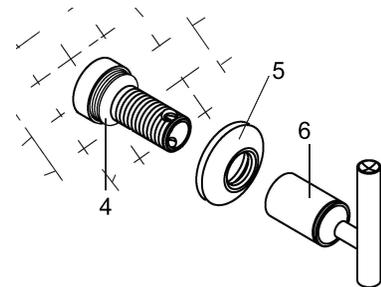
The configuration shown is the correct position of the handles in the closed position.
