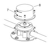
Secure protector(8) onto the base with screws(7).
