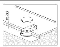
Make sure the distance between bottom of protector and top surface of tiles is within 13~33mm(top surface of tiles is between the MIN and MAX line on the protector). Drill Ø75 hole on the tile. Lay the floor tiles. Cut away the extending part of protector in accordance with the tile surface before installing the faucet. For faucet installation instructions refer to the corresponding installation instructions.
