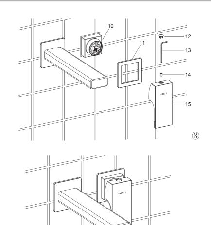
Supply enough plumbers putty or sealant to the rear of the escutcheon(11). Slide the escutcheon with washer onto the valve base(10).
