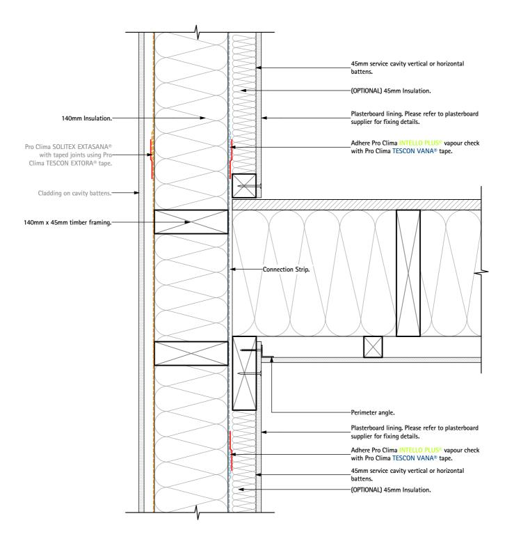
NOTE: Connection Strip must be installed during framing stage.
