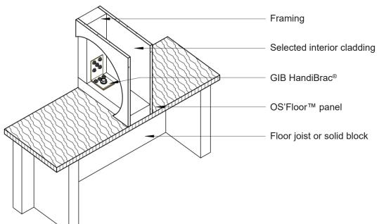
© copyright 2019 IBS Ltd All Dimensions are to be site checked before construction and installation File: rigidrap\_1255 - floor connections **Rigid Air Panel** Reference Scale: Floor Wall Issue: SUSTAINABLE BUILDING PRODUCTS 1 IBS\_1255 p 0800 367 759 www.ibs.co.nz Date: July 2019 **Floor Connections** f 0800 500 549 sales@ibs.co.nz
