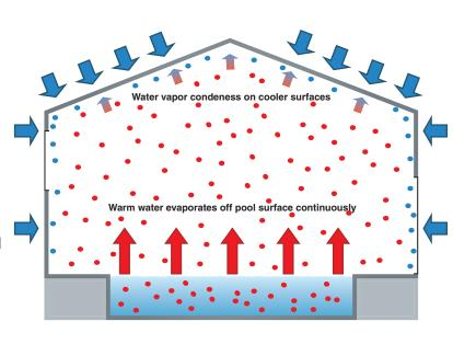
Vent-Air Indoor Pool Ventilation and Heat Recovery Systems are ideal for use in new and existing indoor residential, commercial and public swimming pools, with surface areas starting from 30m<sup>2</sup>.
