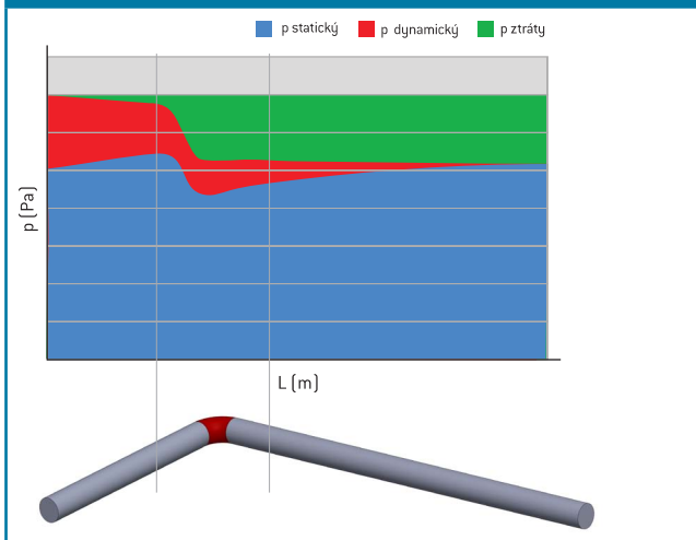
Graph of pressure distribution in a fabric diffuser
