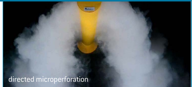
Examples of airflow patterns created through a smoke test in the PRIHODA testing center
