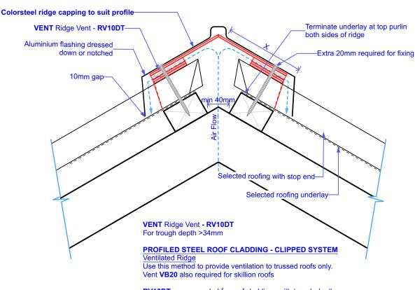
**RV10DT** recommended for roof claddings with trough depth 34mm or greater
