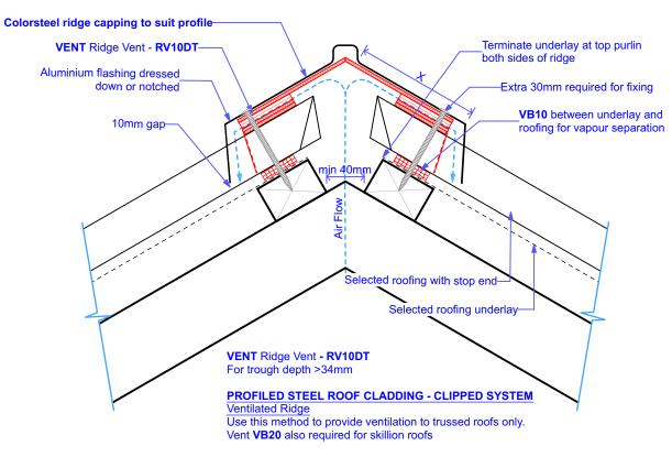
**RV10DT** recommended for roof claddings with trough depth 34mm or greater
