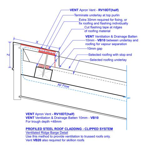
Main contractor to ensure correct placement of purlins for fixing of Ridge Barge Vent
