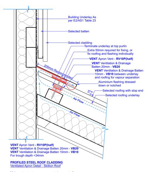
Main contractor to ensure correct placement of purlins for fixing of Apron/Ridge Vent
