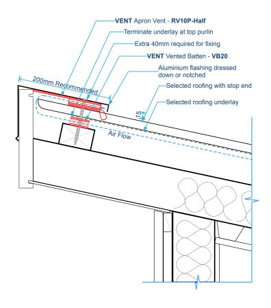
The **VENT Apron or Barge Vent** is created by simply cutting the **VENT Ridge Vent** in half which creates the perfect ventilation product for both abutment or mono pitch barge details. The vents are designed to release warm air from the roof void using the natural convection of rising warm air or by means of negative pressure created by wind blowing over the roof.
