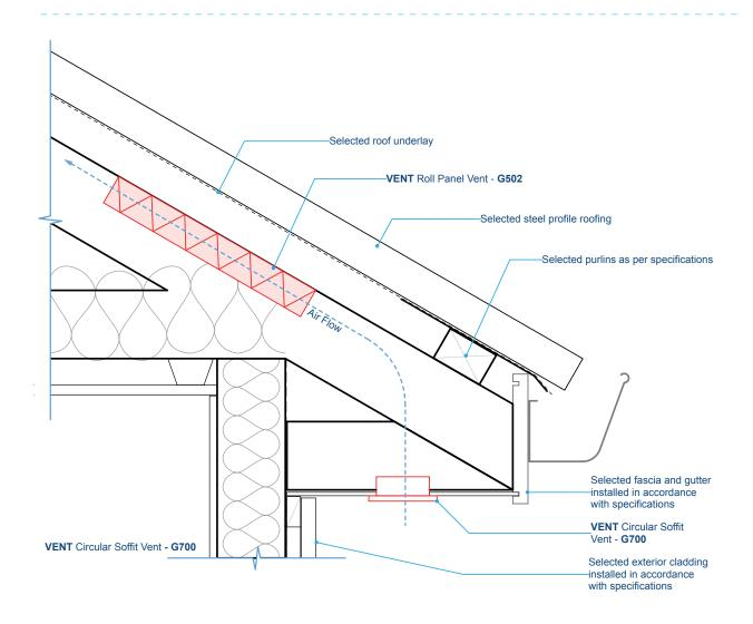
The **VENT Circular Soffit Vent G700** is designed to provide passive airflow into the roof cavity to reduce the risk of moisture build-up.
