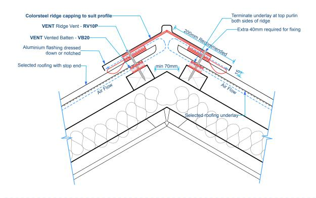
The **VENT Ridge Vent** is designed to release warm air from the roof void using the natural convection of rising warm air or by means of negative pressure created by wind blowing over the roof.
