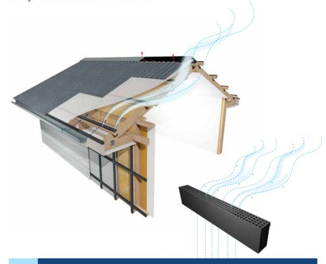
Recommended airflow is determined according to the pitch and the type of roof:
