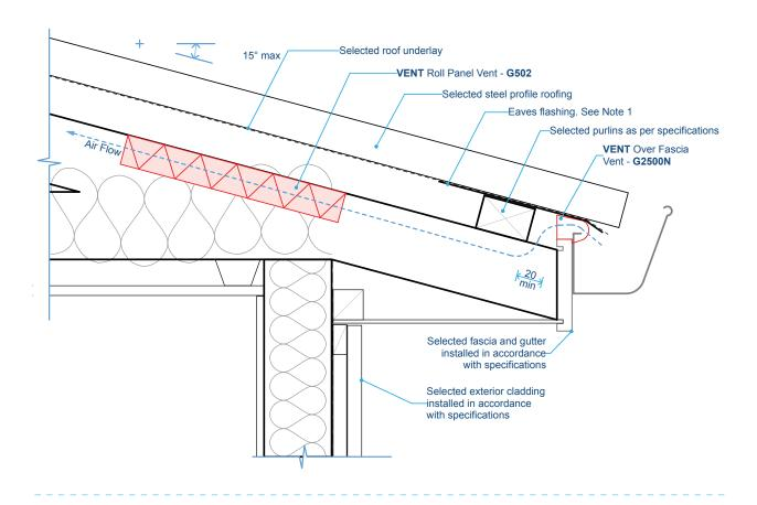
**VENT Over Fascia Vents** are the most practical and cost efficient method of ventilating the eaves. They are easy to install, discrete and are compatible with either timber or metal fascias. Over fascia vents are the only method of achieving eaves ventilation to buildings with no eaves or soffit.
