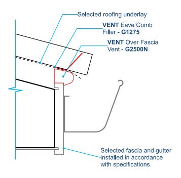
The **VENT Eaves Comb Filler G1275** is designed with flexible fingers which adjust to fill the gaps left when using profiled tiles or steel roof cladding. This prevents entry by birds and large insects beneath the tiles.
