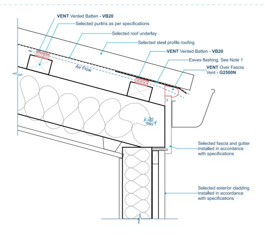
The **VENT Ventilated Cavity Batten - VB20 Roof**, is a strong, durable purlin cavity batten that is designed to ensure that unimpeded airflow of 16,000mm<sup>2</sup> per linear metre is guaranteed through the roof cavity of a skillion roof design, enabling passive airflow around the entire building envelope.
