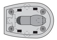
Screw the inside bolt component onto the inside of the door over the Diamond Back Plate.
