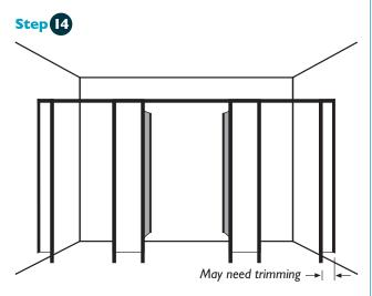
Repeat for the remaining Stiles and Fascias. Check the last Fascia before fixing as it may need trimming.
