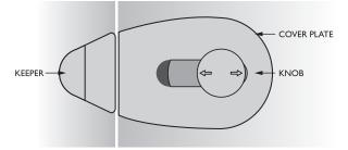
Then clip on the cover plate. Push on the knob and tighten the grub screws with the allen key supplied. Finally Fix the keeper on the fascia.
