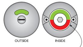
Insert the green and red plate into the inside of the front component of the indicator bolt.
