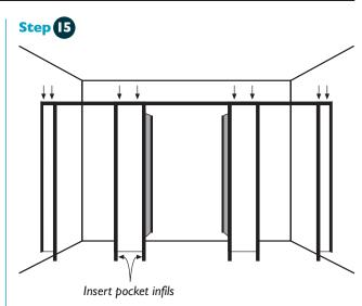
Fix Fascia panels in place, screw fix Headrail into the top of the full stiles.
