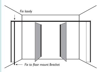
Headrail connecting into the Full Stile. (Not to scale).
