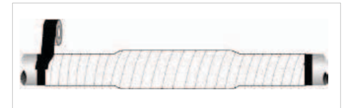
Fig. 18-13 Wrapping the protection area with black/grey tape
