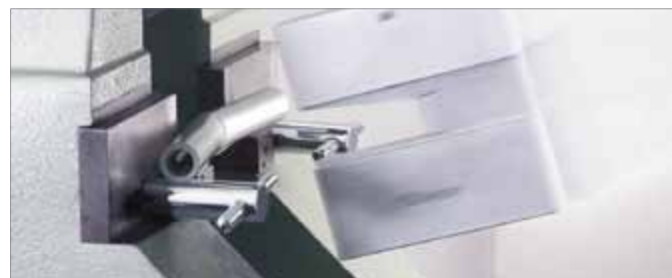
Fig. 3 - 2 Universal pipe RAUTITAN flex in the notch impact testing device
