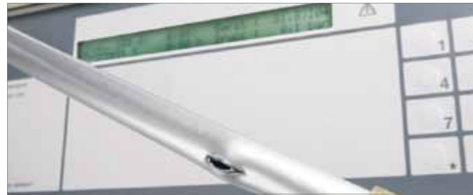
Fig. 3 - 1 Result of a burst pressure test with the universal pipe RAUTITAN flex
