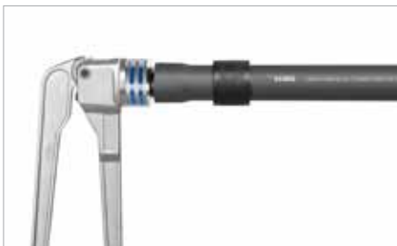
1. Expand the pipe x2 (rotate 30°)
