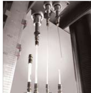
Illustration 2-7: Tensile-strength testing procedure
