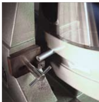
Illustration 2-6: RAUTITAN flex universal pipe in impact-testing device
