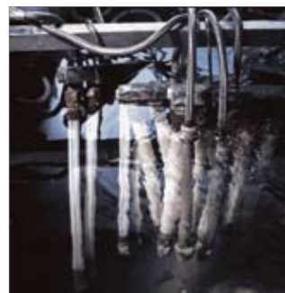
Illustration 2-8: REHAU pipes in endurance testing (under pressure in water basin)
