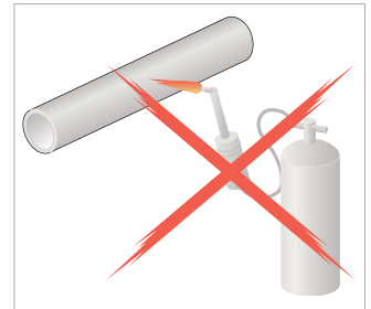
Illustration 2-79: Protect pipes from excessive heat
