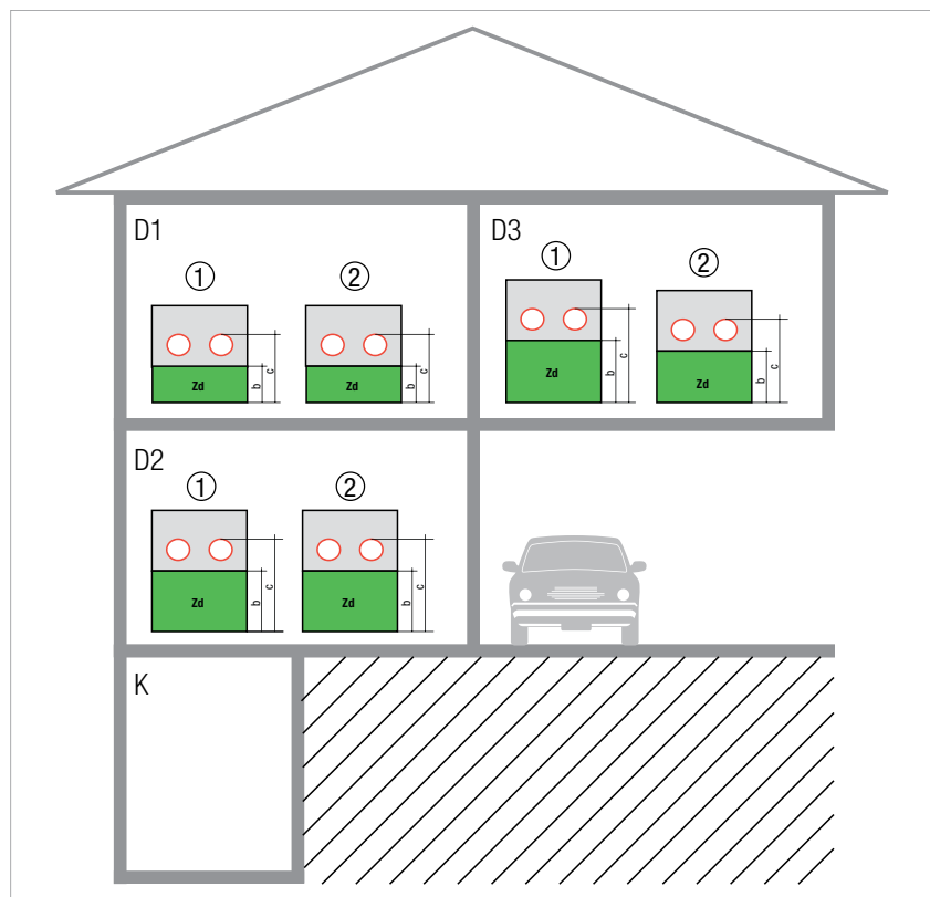
Illustration 4-53: Minimum insulation layer constructions with the REHAU pipe grid system
