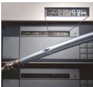
Illustration 2-5: Result of a burst test with RAUTITAN flex universal pipe
