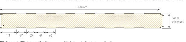
Rib External / Rib Internal Profile
