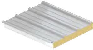
KS1000RW Trapezoidal Roof Panel is a through fix insulated panel, with a trapezoidal profile and 1000mm cover width, allowing for fast track and cost effective installation on all building types. Standard specification is suitable for roof slopes 4° and above (after deflection) – alternative specifications available include high humidity, low temp and low pitch (min 3°).
