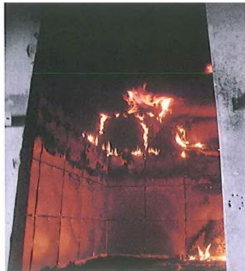
Fire in room corner test according to ISO 9705
