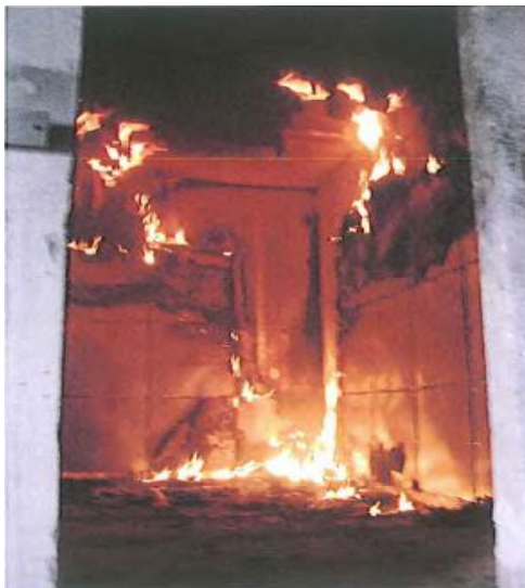
Fire in room corner test according to ISO 9705
