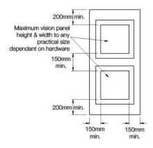
The standard glazing system provides a flush attack face and steel beading with fixings on the "non-attack" face. Glazing with ballistic rating G2 is available.
