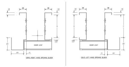
Note: Frame shown with optional folded steel stop to receive lock.
