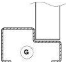
Steel frames require packing of the frame during installation with fibrous insulation material (e.g. fibreglass, mineral wool or polyester batts).
