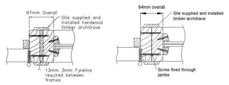
\* For the VP60 system, the separate glazed sidelight is connected to the fire door frame with a layer of 13mm plasterboard between. The joint is covered by a timber architrave as illustrated above.
