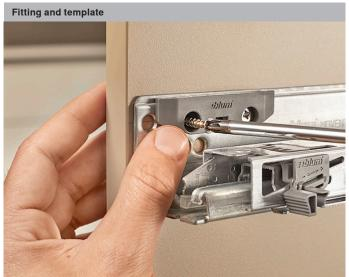
The locking unit and latching element also serve as a template. Place the screws in the predefined fixing positions. You can use either chipboard or system screws for fixing the latching element.
