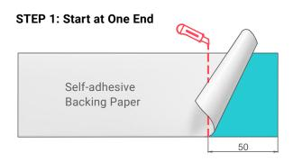
Peel back 50mm of backing paper at one end and cut off with a utility knife. Position the exposed self-adhesive surface on the substrate and lightly apply pressure. Check that all the edges line up.
