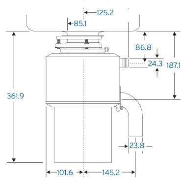
NOTE: Plumb 38.1 mm waste line to prevent standing water in disposer motor housing.
