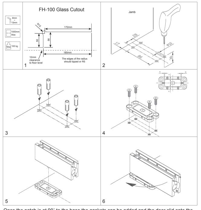
Once the patch is at 90° to the base the gaskets can be added and the door slid onto the patch and clamped in place by tightening up the screws on the side. The door speed and brake speed can then be adjusted to suit your requirements, then the cover caps clipped in place to complete the installation.
