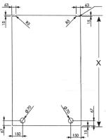
X = height of door which is finished opening height less 35mm
